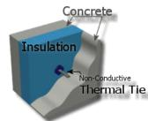
Tilt-up is a much tighter building system than traditional methods; an R16 Tilt-Up
